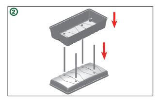
Install vertical pipes, and Install body of case well with vertical pipes.
